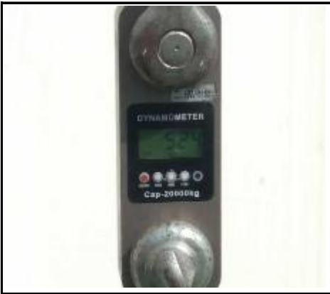
Loading test over 5 tons(the capacity of the crane is 4 tons)
