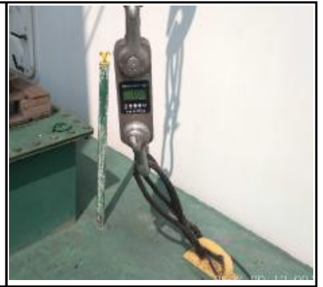
Loading test after repair (two places)
